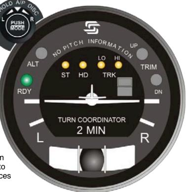
The TC component of the autopilot operates exactly as the instrument it replaces, complete with a red flag indicating that electrical power to the instrument has been lost. The TC powers up along with the battery master as usual.
